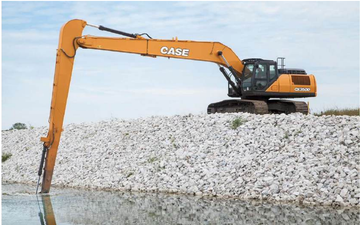
Photo 3 - Long Reach Excavator
