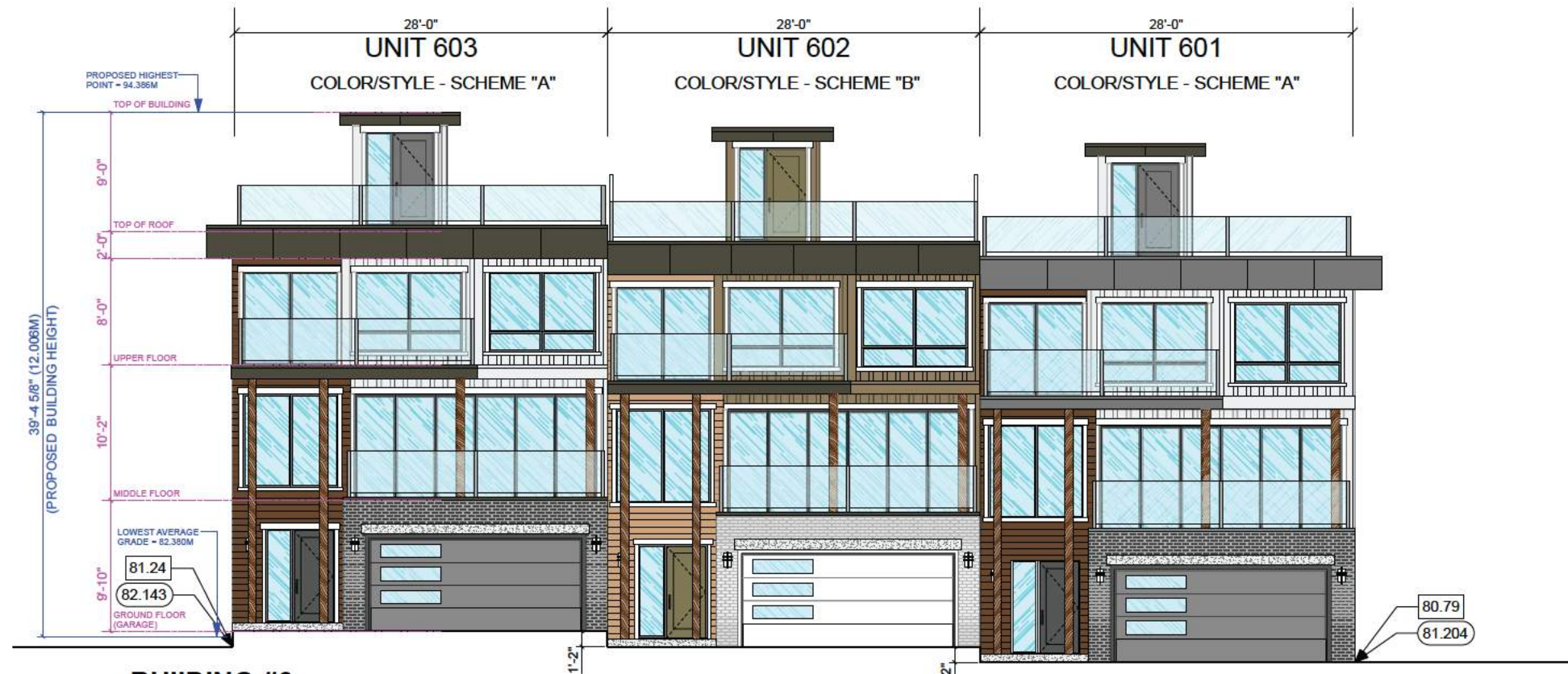
BUILDING #6 FRONT ELEVATION (EAST)
