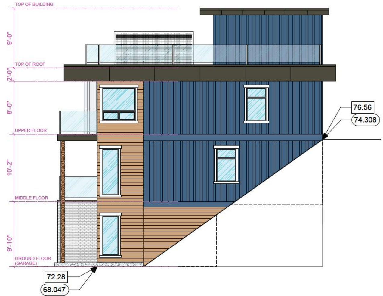
SIDE ELEVATION (NORTH)
