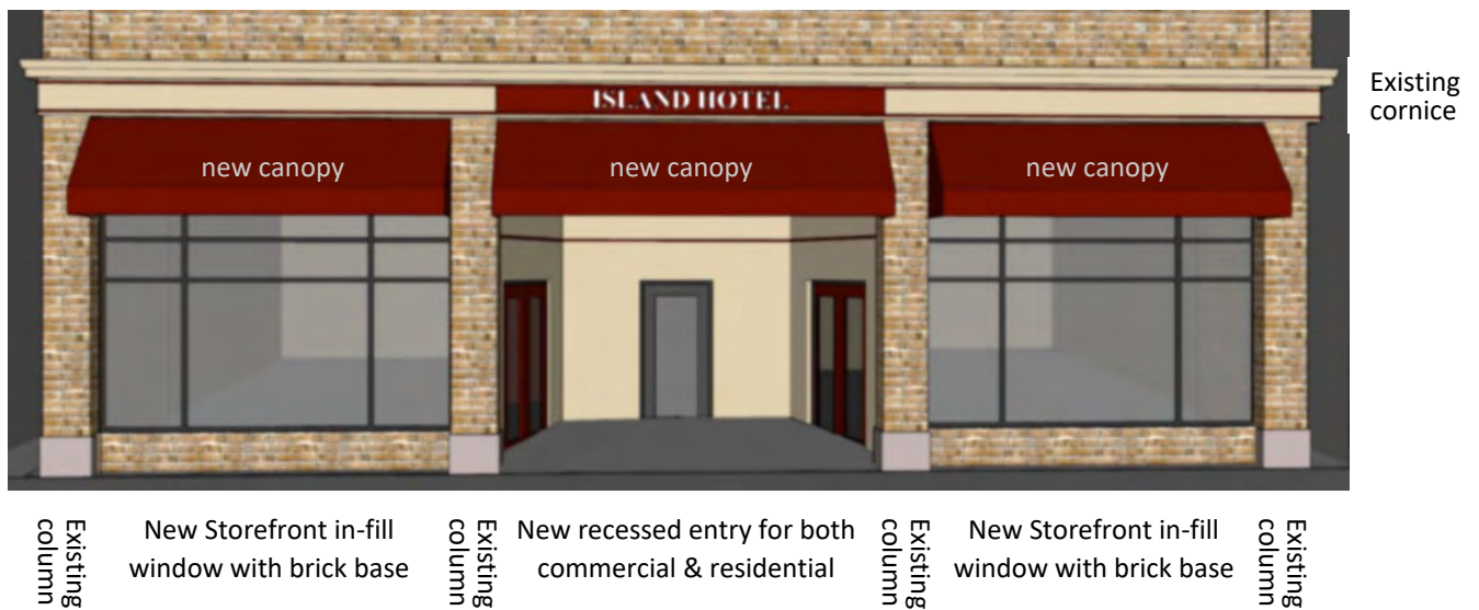
Front Elevation Renovation - Concept
