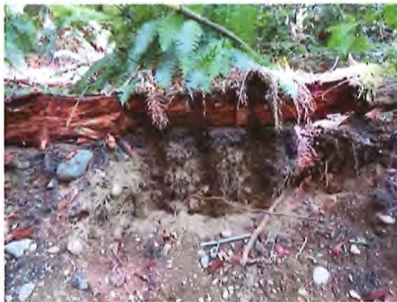
Soil Profile Lot 13. The site is characterized by well-drained gravelly sandy soils.
